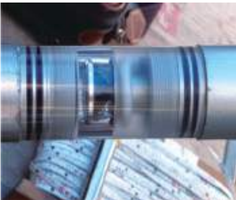
Fig. 5.11: Use of bore hole camera to study bore wall
