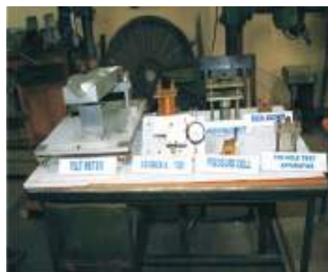
Fig. 5.6: Indigenous instruments (Tiltmeter, Crackmeter, Pressure Cells) for slope monitoring
