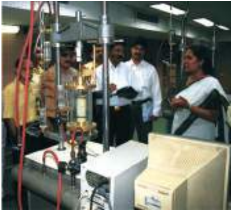
Fig. 5.1: Triaxial Test apparatus for evaluating strength parameters
