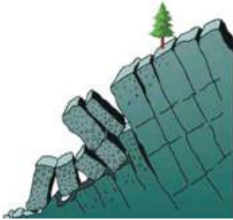
Fig. 1.4: Sketch showing the end-over-end motion of rock down a slope during toppling
