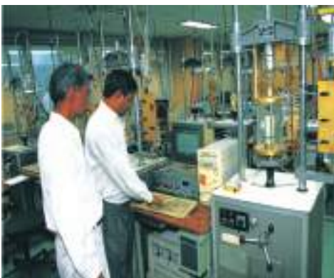
Fig. 5.5: Computer Controlled Triaxial Test Equipment
