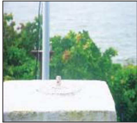
Fig. 6.14: Permanent station used to monitor movement using peg markers
