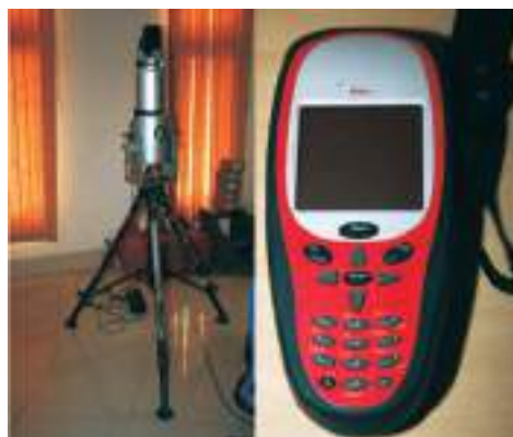
Fig. 6.12: Hand held GPS and Total Station
