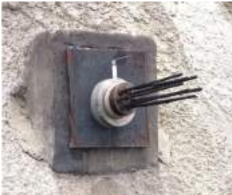
Fig. 7.33: Multi-bar reinforcement with an instrument to record wall pressure
