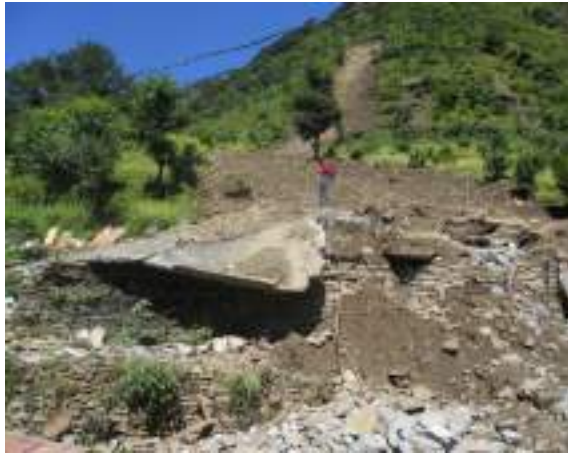
Fig. 35. Photograph showing damaged agricultural fields and houses due to rock cum debris slide.
