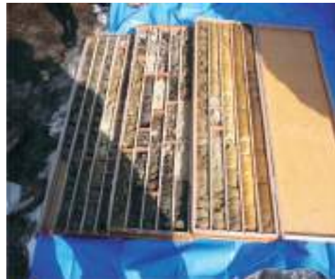
Fig. 5.12: Core logs used to identify and grade subsurface materials
