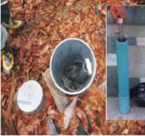
Fig. 6.1: Inclinometer used for monitoring subsurface displacement
